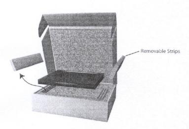
1. Remove instruction sheet, tape strip and 1/2" foam from interior of box. If necessary, remove foam tear-out strip(s) along sides and back edge to accommodate larger laptops. A snug fit is desirable.
